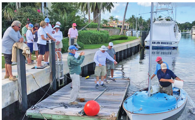
This test, set up by George Lucas, showed that with air bags installed in our sailing vessels, the Bullseye will not sink when it's filled with water.
