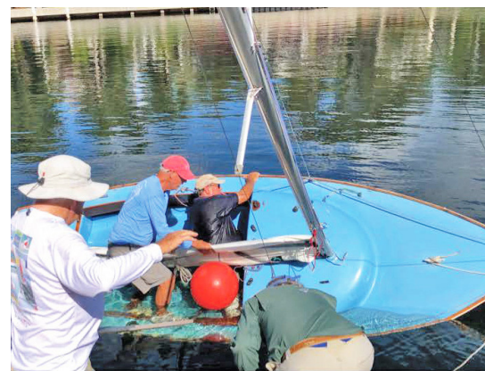
This test, set up by George Lucas, showed that with air bags installed in our sailing vessels, the Bullseye will not sink when it's filled with water.
