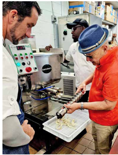
Gianni Chef de Cuisine Ryan Schmidt and Emilio Miti clean the auger that forced the pasta dough through the forming die.
